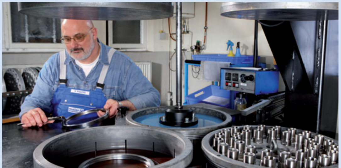
Lapping of sealing surfaces
